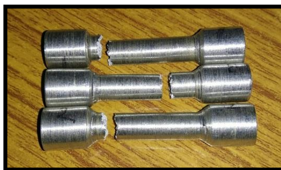
Figure 4.2: Tensile Specimens After Test
